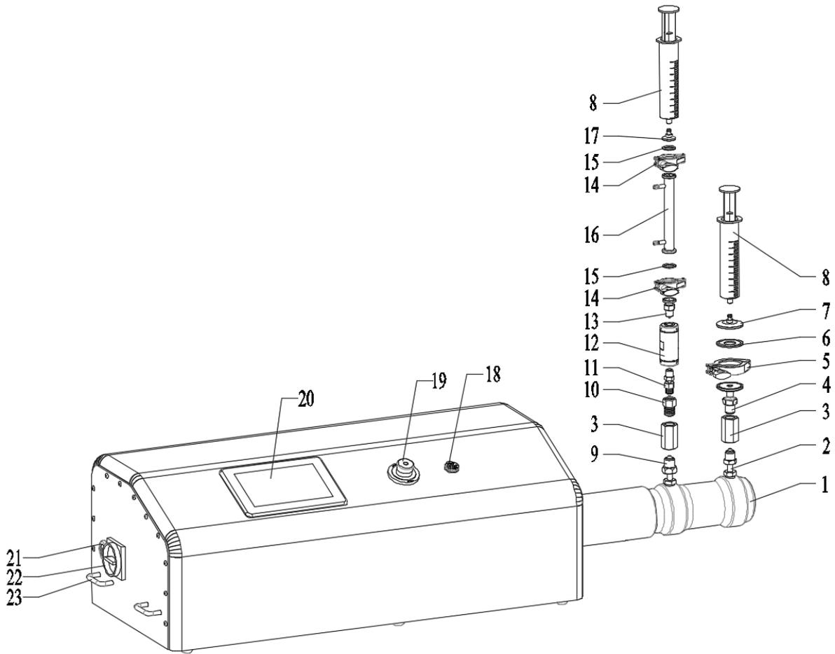
**General Arrangement Drawing of UltraGenizer with Heat Exchanger Optional**
